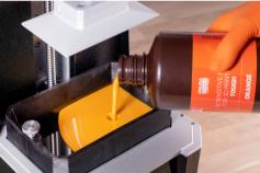
Tighten both screws simultaneously and with the same amount of force. Pour the recommended amount of resin - there is a max level mark in the tank.
