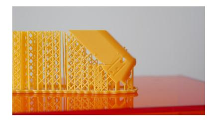
**Solution:** Try printing a sample object and see if the issue persists. If it does, clean the resin tank properly and try again. Continuous issues with separated / missing layers can be caused by a faulty UV LED panel - check whether it works correctly. Otherwise, the cause is most likely a broken object file. Either try re-slicing the model or download a new one.
