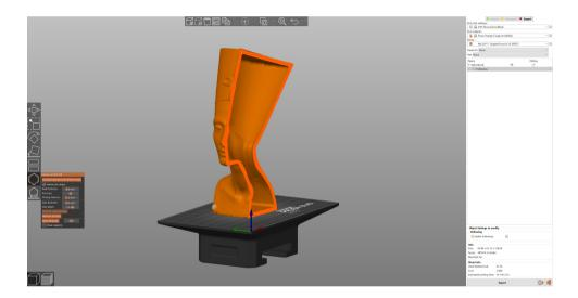
Hollowing can be configured for each model individually using the Hollowing tool in the left toolbar. Alternatively, you can configure hollowing for all models at once in *Print Settings - Hollowing*.
