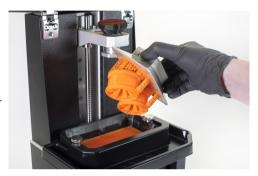
Use the **bundled metal spatula** to remove the print from the print platform. To prevent injuries, **do NOT use your fingernails** to remove the prints since the plastic can easily get under your nails and break off.
