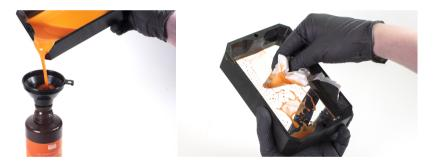
Use the bundled funnel with a filter to pour used resin into a bottle (don't mix old and new resins).
