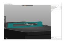
Insufficient amount of supports - the orange colour shows a single layer that the printer is going to cure and then attempt to separate from the bottom of the tank. The single support can't withstand the peeling forces. This usually happens if you set the support density to extremely low numbers.
