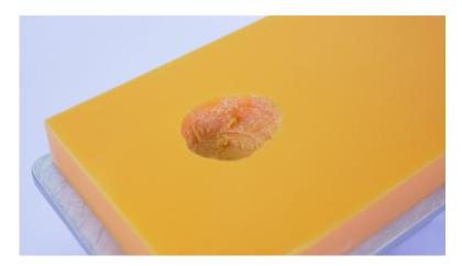
**Solution:** Make sure the FEP foil on the bottom of the tank is perfectly clean. Carefully remove any dirt / solidified bits. If the FEP foil is cloudy, use hot water and dishwashing soap to clean it and restore it to the original look.
