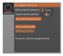
In the picture on the left is the **SLA Support Points** menu, which can be found in the left-side toolbar. If you can't open it, it usually means the model you have imported is too large for the print bed. Move, rotate and scale the object so it fits - the object should be displayed in green colour.
