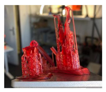
**Solution:** Make sure the printer is properly calibrated, tighten the black knob at the top of the tower and tighten both resin tank screws evenly and with the same amount of force.
