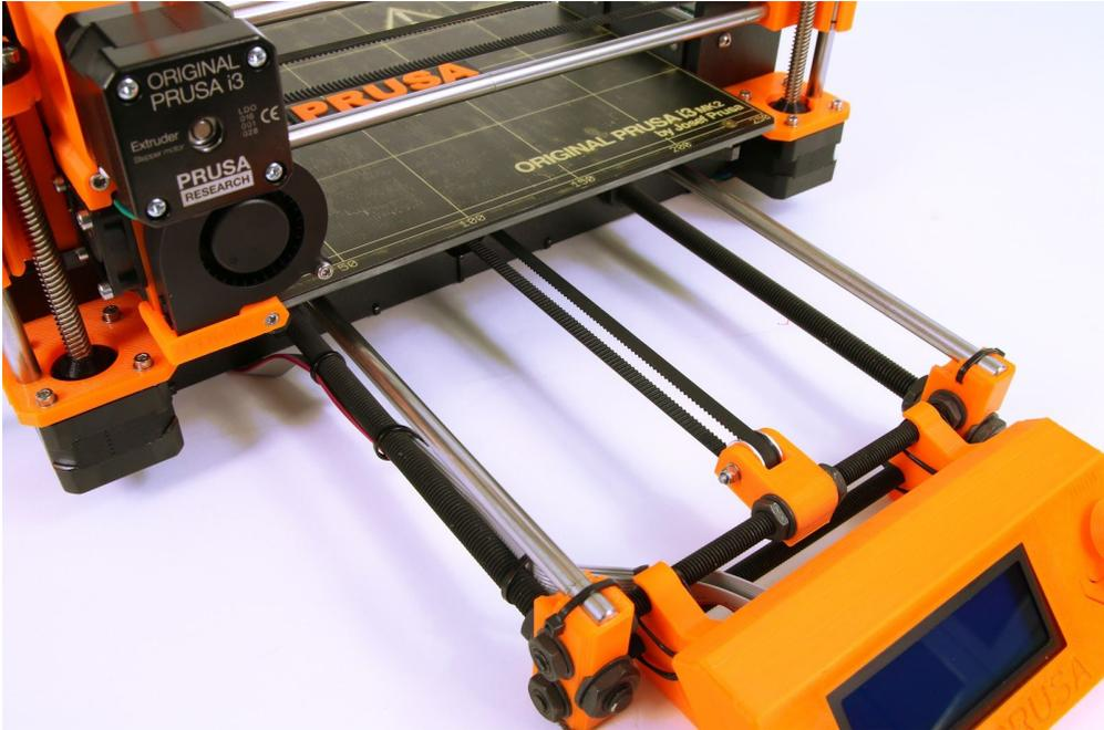
*Pict. 47 - A properly tightened Y-axis belt under the heatbed*
