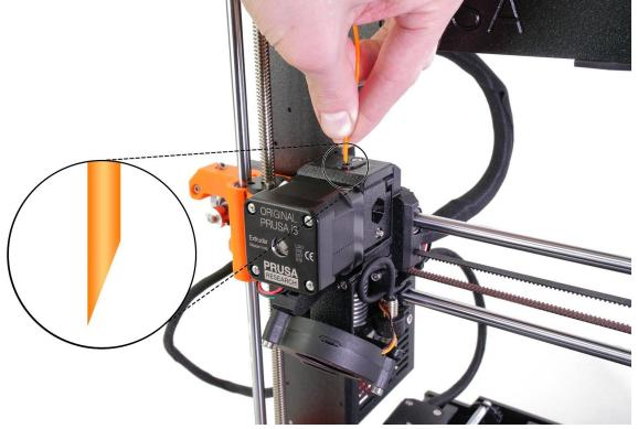
Pict. 9 - Loading the filament into the extruder
