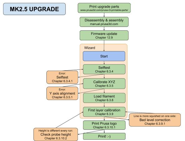
With your first start-up of your freshly-assembled printer, it will guide you through all the tests and calibrations you need to do to get started printing. Wizard can be also started manually from **LCD menu - Calibration - Wizard**. Do not forget to read chapter <u>6.2.2 Flexible steel</u> <u>sheet surface preparation</u> before running the Wizard.
