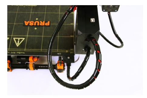
Pict. 49 - Cables should be wrapped in a spiral wrap
