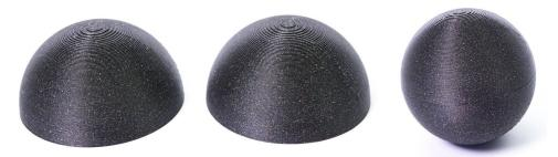
Pict. 29 - A sphere printed in two seperate parts glued together
