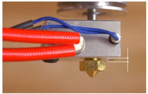
Pict. 41 - A gap between a fully screwed in a nozzle and the heater block
