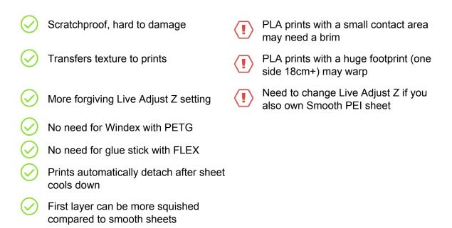
Powder coating directly on metal makes it very hard to damage this build plate. If a heated nozzle crashed into it, the metal can dissipate the heat. Powder coating also gives the surface a distinct textured look that will be visible on your prints.
