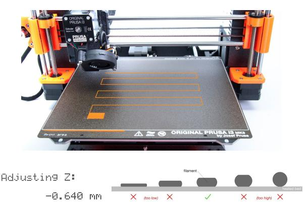
*Pict.* 10 - How to tune the nozzle height live during the test print. Note: -0.640 mm is only for illustration. Your setting will be different!
