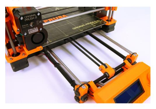
Pict. 47 - A properly tightened Y-axis belt under the heatbed
