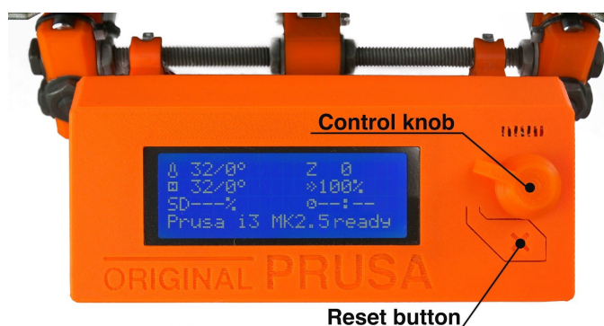
Pict. 16 - LCD screen and control buttons
