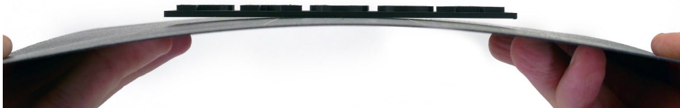
Pict. 14 - Removing the model from the PEI print surface by bending the steel sheet. If the prints still do not want to get loose or you need to bend the sheet too much (which you should not do), try to bend the sheet inwards.
