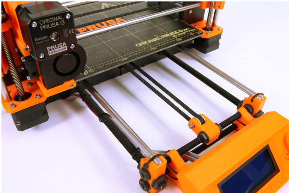
Pict. 44 - A properly tightened Y-axis belt under the heatbed
