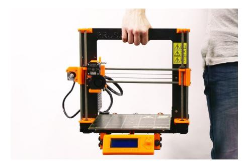
Pict. 3 - Proper handling of a printer
