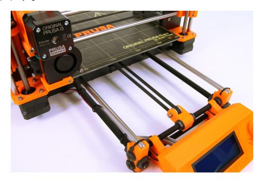
Pict. 38 - A properly tightened Y-axis belt under the heatbed
