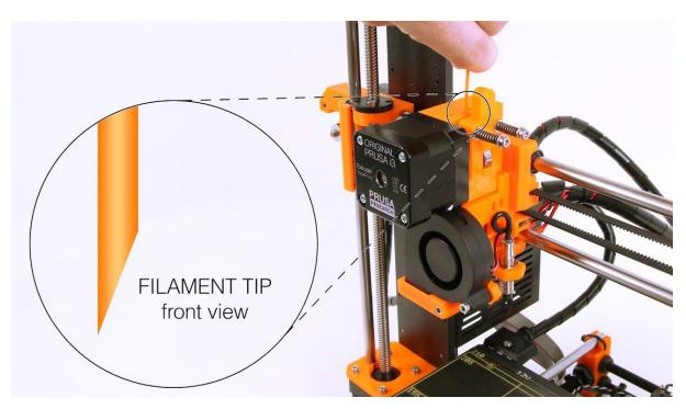
Pict. 7 - Loading the filament to the extruder
