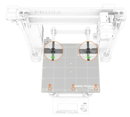
Pict.21 - Example in the picture - moving the frame forward on the Y axis (increasing the 100 mm distance from the build manual) will increase the Y distance from min.
