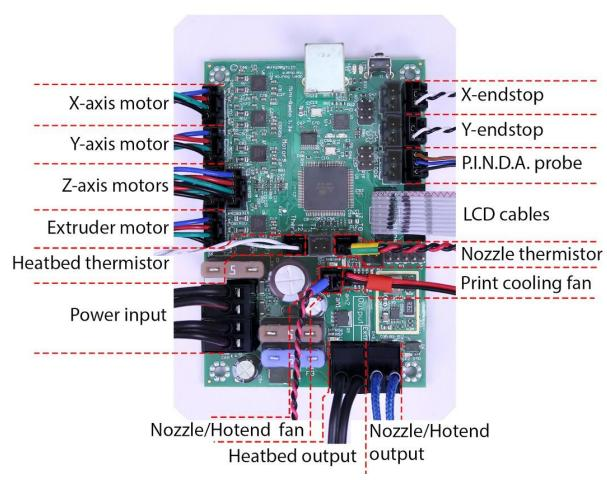
Pict. 37 - Proper wiring of the connectors
