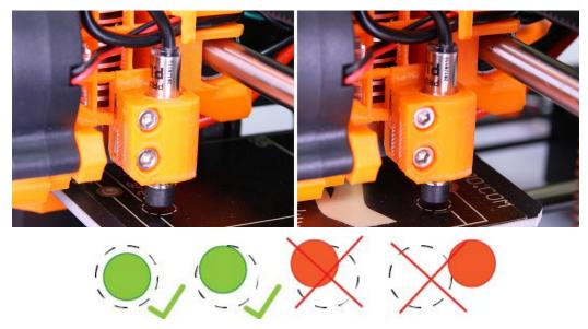
Pict. 6 - The probe must be inside the circles (1st and 9th calibration point) to successfully level the bed.
