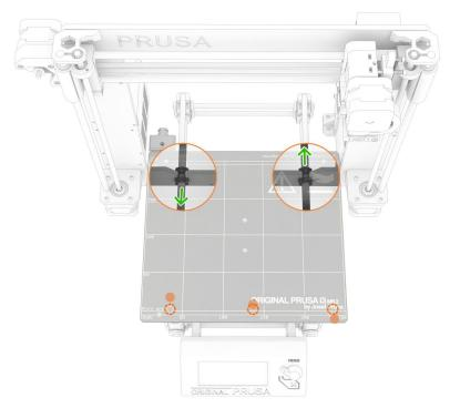
Pict. 22: moving one side of the frame forward (increasing the measured value) on the Y axis and other side backward (decreasing the measured value) according to the values from the first screen will improve the skew.
