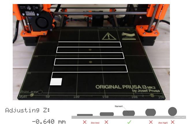
Pict. 8 - How to tune the nozzle height live during the test print. Note: -0.640 mm is only for illustration. Your setting will be different!
